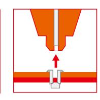
4. Close the handles to rivet, then exit the riveter.
