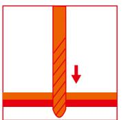
1. Drill a suitable hole in the two needed riveting metal.
